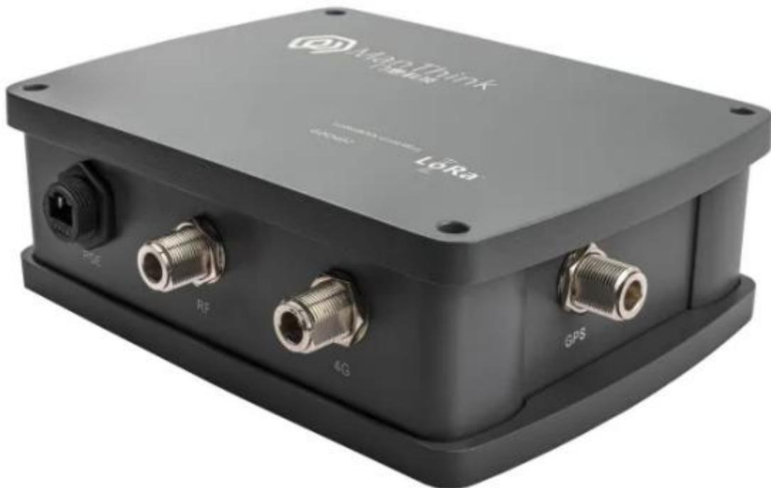
GDO31X shell adopts die-cast aluminum structure, which is simple and thick, with strong oxidation resistance and good waterproof and dustproof performance. The external antenna adopts RF N-type connector, which has high reliability, strong vibration resistance and excellent mechanical and electrical properties. POE interface adopts customized RJ-45 waterproof connector, giving consideration to reliability and convenience.
