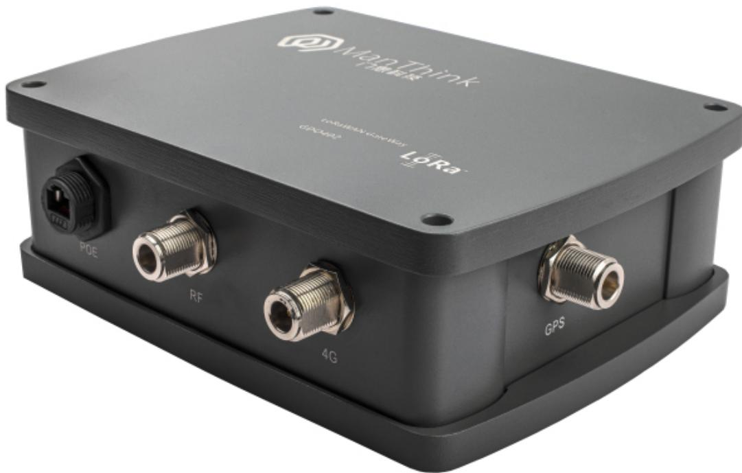
GDO318 shell adopts die-cast aluminum structure, which is simple and thick, with strong oxidation resistance and good waterproof and dustproof performance. The external antenna adopts RF N-type connector, which has high reliability, strong vibration resistance and excellent mechanical and electrical properties. POE interface adopts customized RJ-45 waterproof connector, giving consideration to reliability and convenience.
