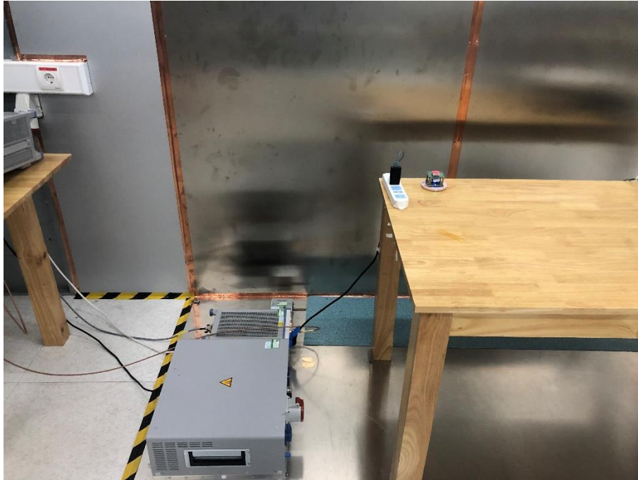
Photograph 1: Set-up for Conducted Emission on AC Mains
