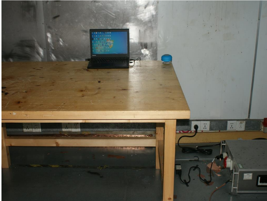
Photograph 1: Set-up for Conducted Emission on AC Mains
