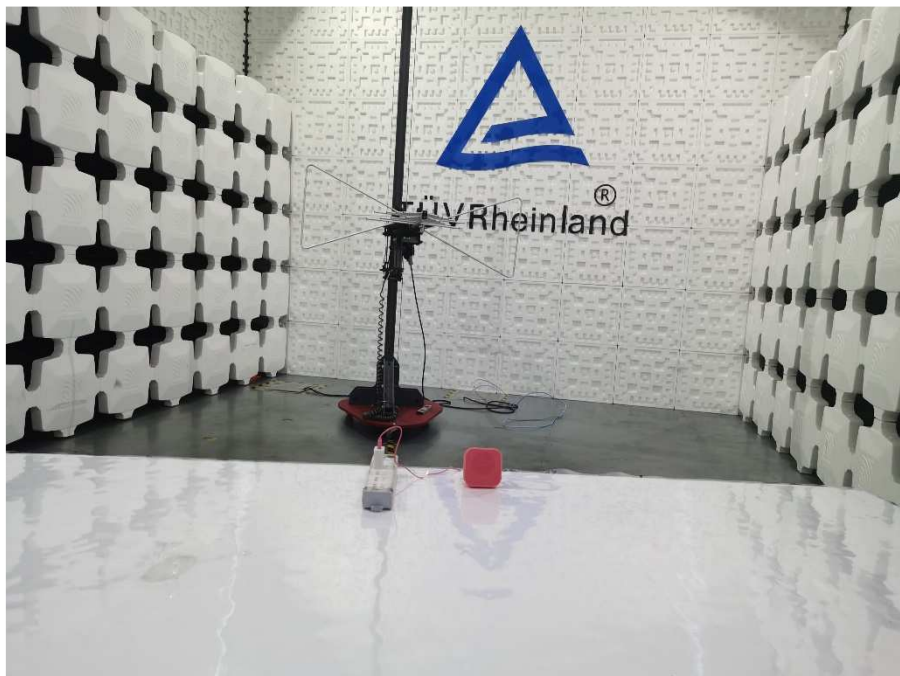
Photograph 4: Set-up photo for Radiated Emission, Below 1GHz
