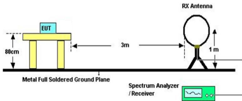
In 3m Anechoic Chamber Test Setup Diagram for 30MHz-1GHz
