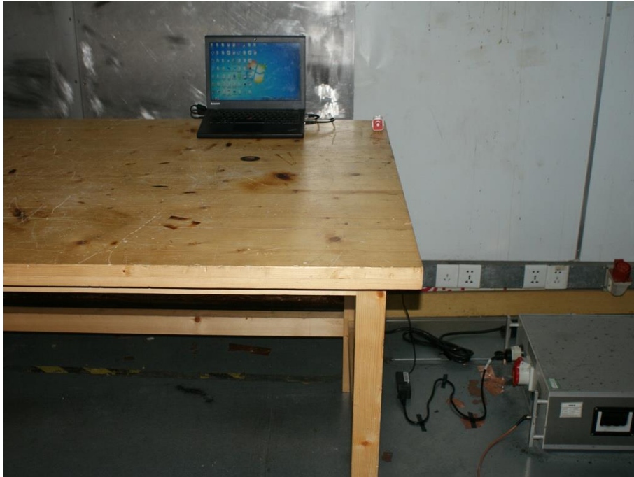
Photograph 1: Set-up for Conducted Emission on AC Mains
