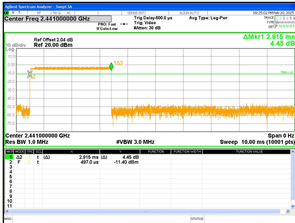
Dwell NVNT 3-DH5 2441MHz Ant1 Accumulated
