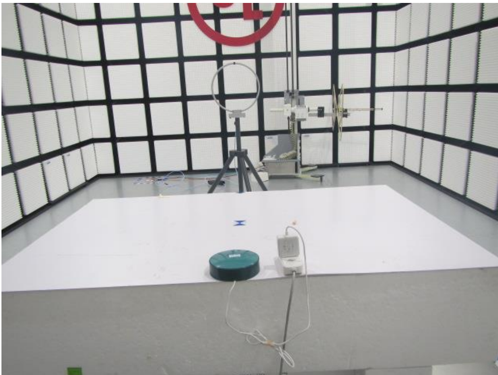
RADIATED DISTURBANCE ABOVE 30MHZ MEASUREMENT SETUP FOR SUB 1GHZ
