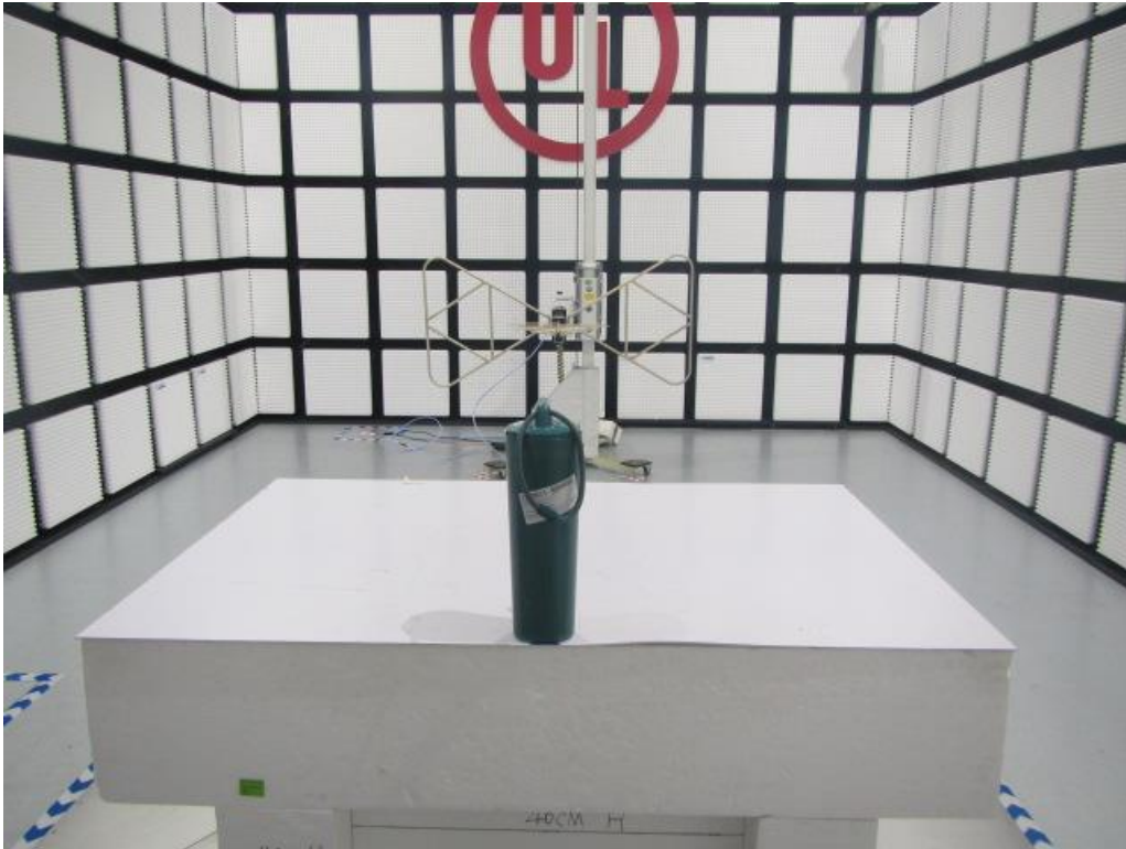
RADIATED DISTURBANCE BELOW 30MHZ MEASUREMENT SETUP
