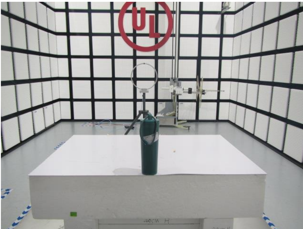
RADIATED DISTURBANCE BELOW 30MHZ MEASUREMENT SETUP
