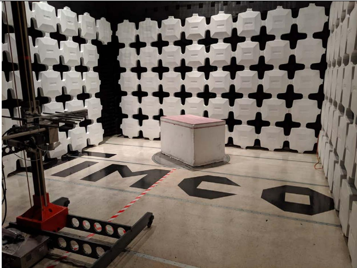
**Radiated Emissions Above 1 GHz Setup, Occupied Bandwidth / Bandedge**
