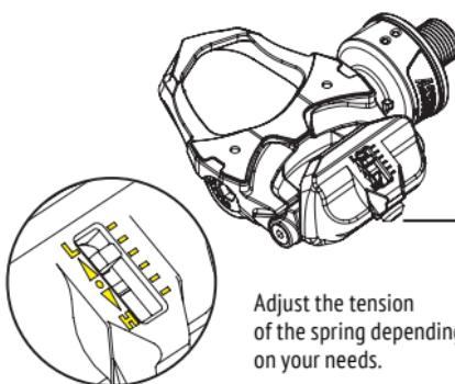
The spring tension can be adjusted using the screw shown in the picture. To increase the tension turn clockwise; to decrease the tension, turn counter-clockwise. Use a 3 mm wrench (not supplied).
