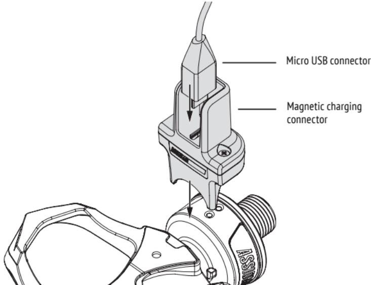
**To charge the batteries, follow the procedure below for each sensor:**
