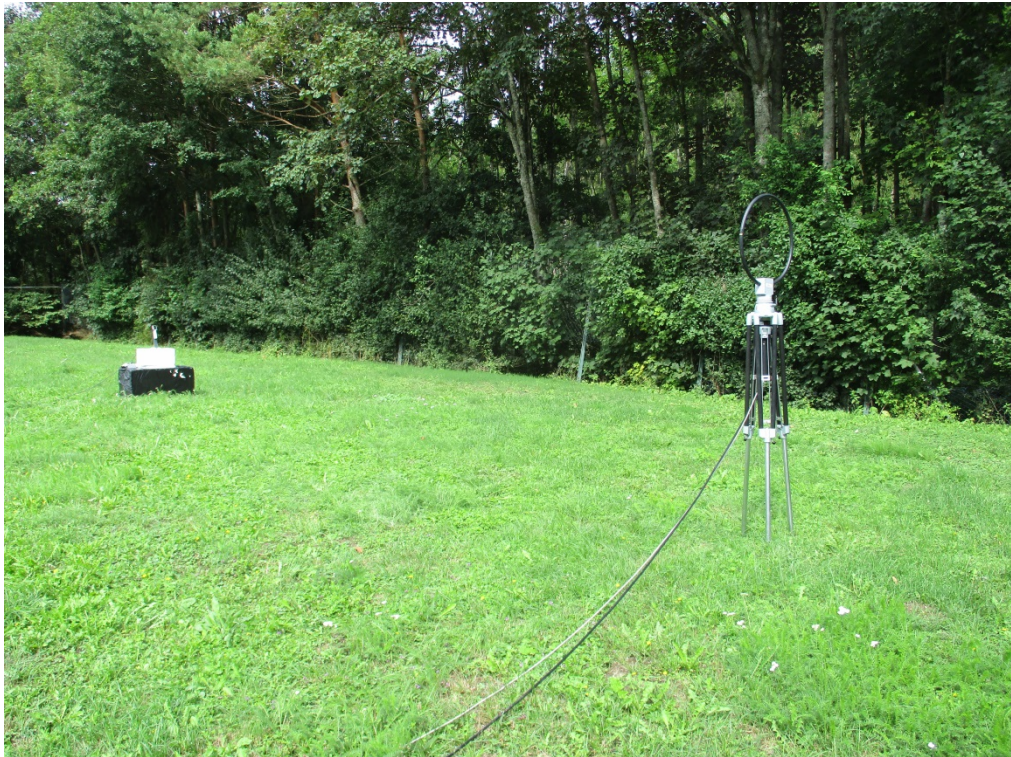
Photograph A1-3: Radiated Emissions 9 kHz - 30 MHz at 10 m distance at open field site
