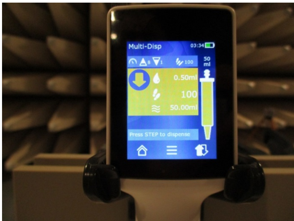
Photograph A1-10: Detailed setup of dispenser in multi-dispense mode
