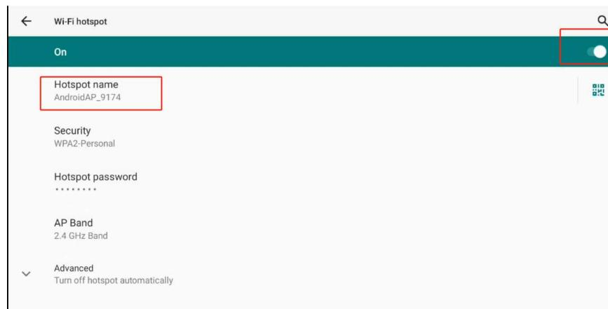
6、Use the test computer or tablet to find the product's mobile hotspot and link it, if it can be linked, the hotspot function test is passed.
