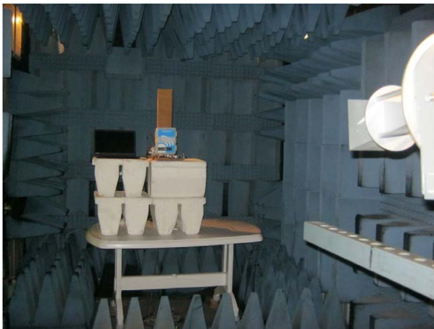
Figure 9. Radiated Emission Test, 18-26.5GHz
