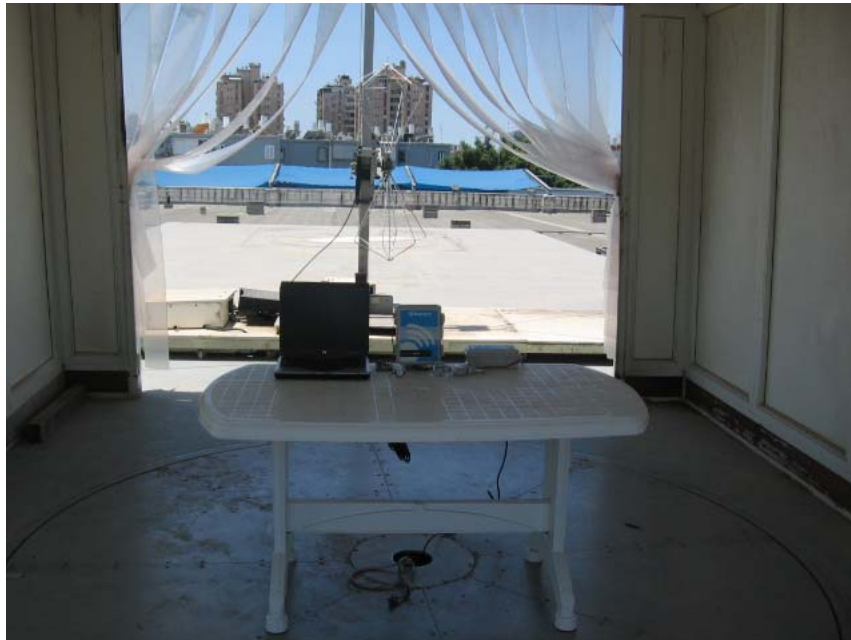
Figure 6. Radiated Emission Test, 30-200MHz
