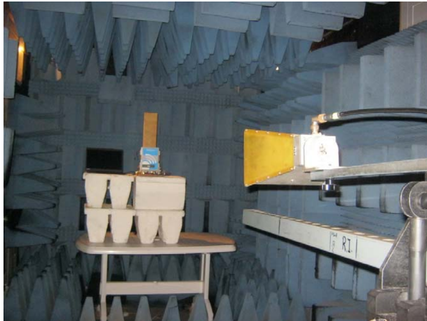
Figure 8. Radiated Emission Test, 1-18GHz
