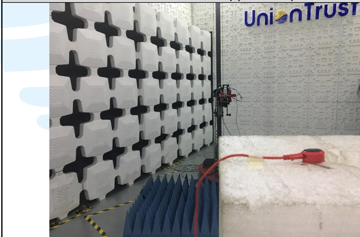
Radiated emission Test Setup (Above 1 GHz)
