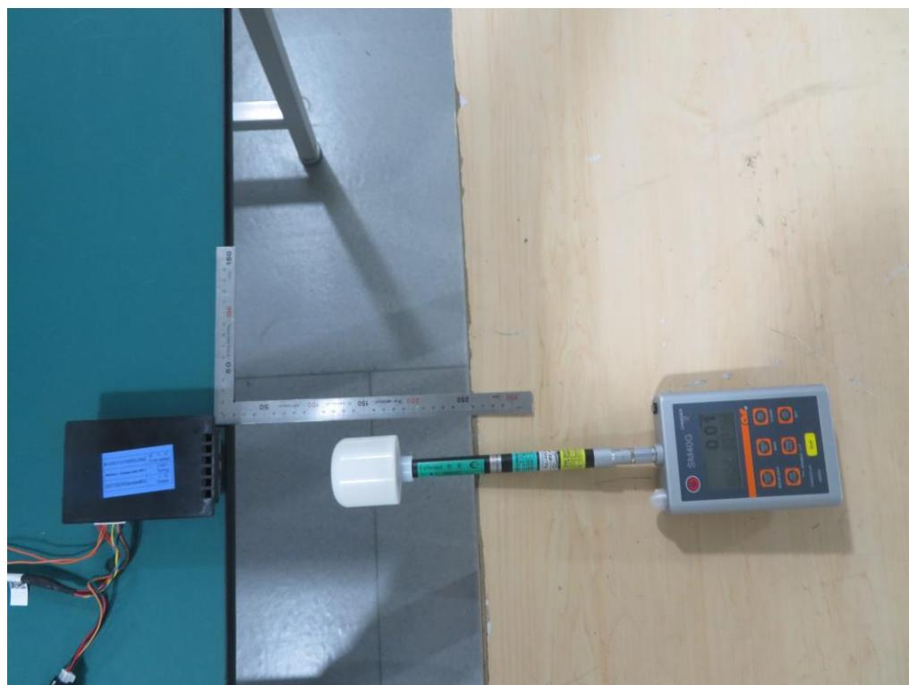
Description: RF Exposure Test Setup for Magnetic Field Emissions
