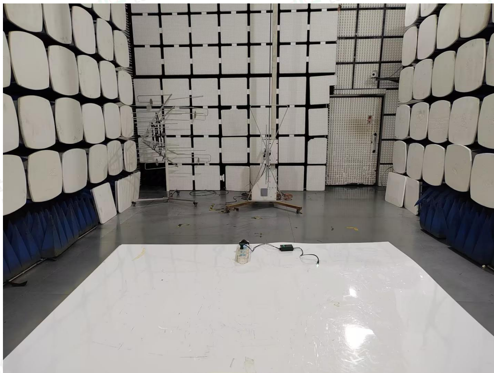
Test Setup Photo(s) of Radiated Emissions Measurement
