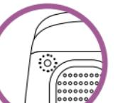
Connect the charger, and a white light will flash while the charging is in progress.
