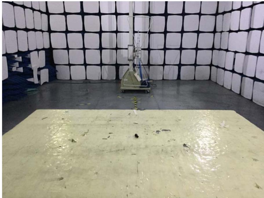
**Radiation Emission Test Setup (1GHz to 18GHz)**
