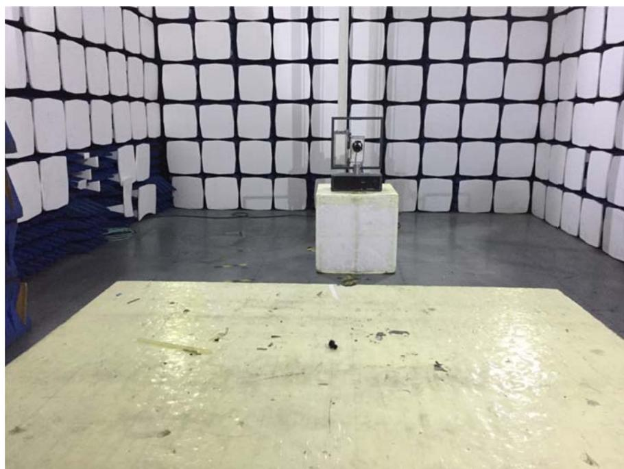
**Radiation Emission Test Setup (30MHz to 1GHz)**
