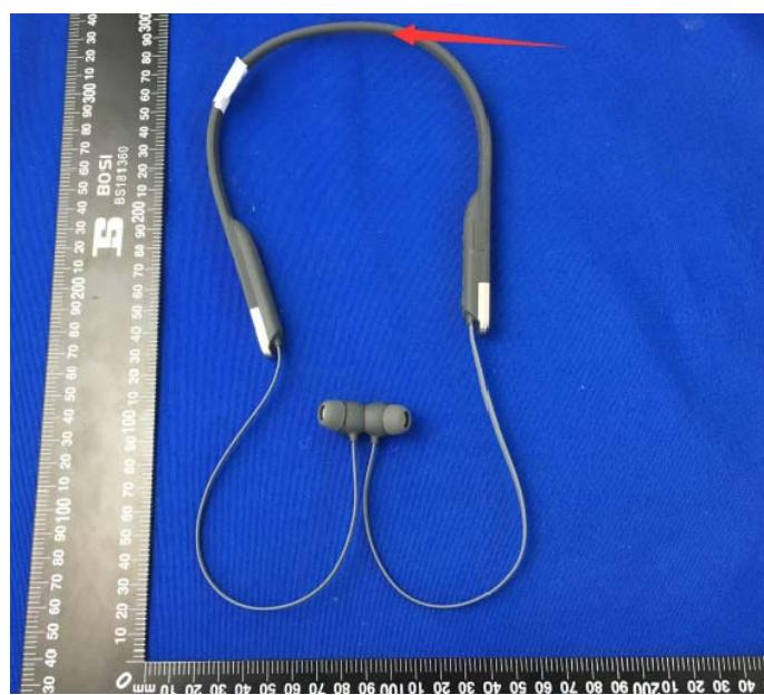
There are limited room to place the whole cert information and surface of earbud is so smooth that we can not place message on it, so we just use tags to show the whole cert message. The material of tags is anti-fire and can not be tear easily when normal used.
