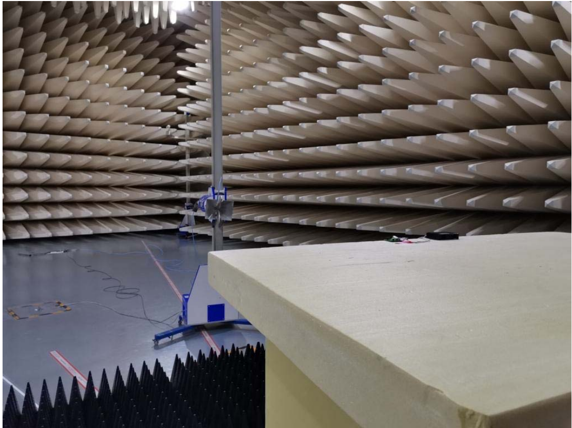
Radiated test setup
