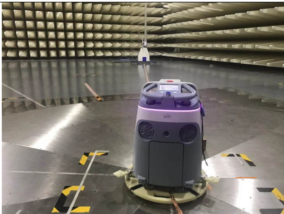
Spurious Radiated Emissions Test setup (30-1000MHz)
