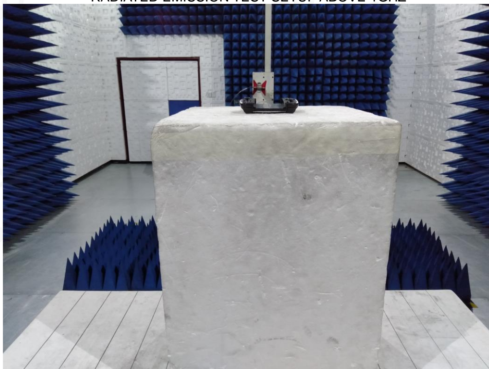
RADIATED EMISSION TEST SETUP ABOVE 1GHZ
