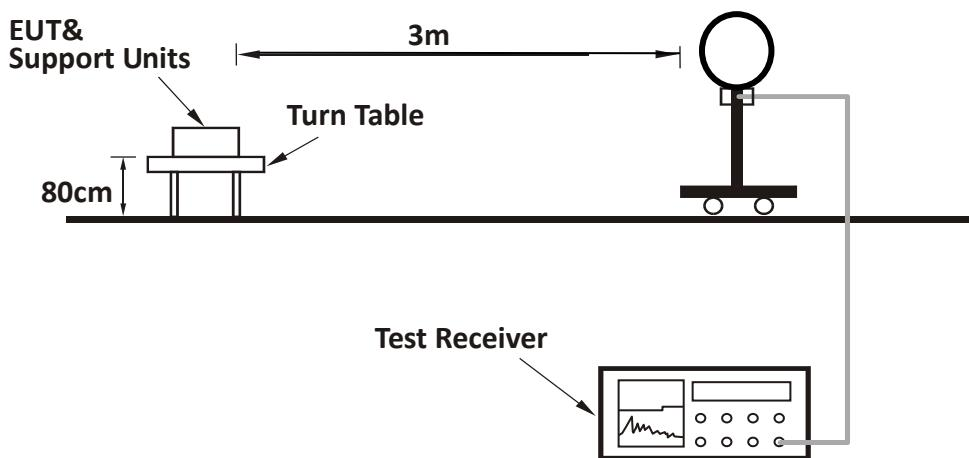
**For Radiated emission 30MHz to 1GHz:**
