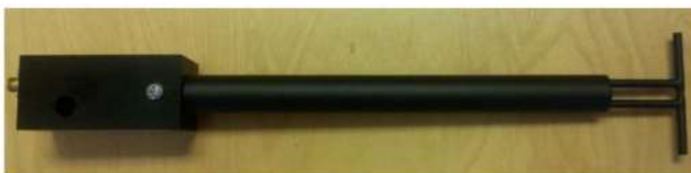
Figure 1 – MVG COMOSAR Validation Dipole
