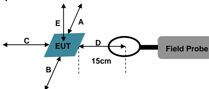
**Remrak:** The E300 probe antenna diameter is 15cm.
