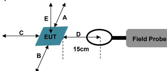
**Remark:** The E300 probe antenna diameter is 11.5cm.
