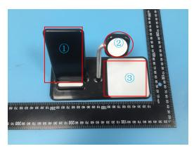
① Wireless charging area which has two charging coils. One coil is working, the other one is stop.
