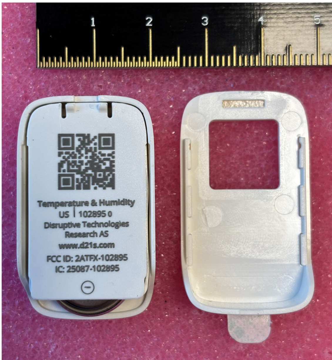
Figure 2: Picture of the back side of 102895 - Wireless Temperature and Humidity Sensor US with the mounting bracket removed.
