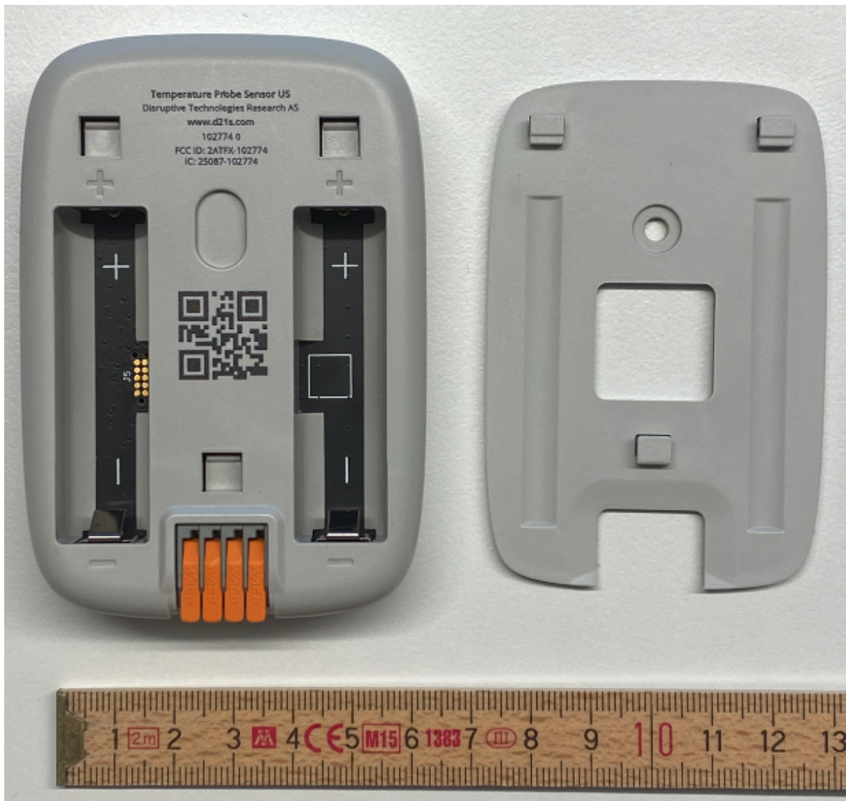
Figure 3: Picture of the backside of 102774 - Temperature Probe Sensor US. The wall bracket is placed on the right side of the sensor with the side intended to be mounted on the wall facing down.
