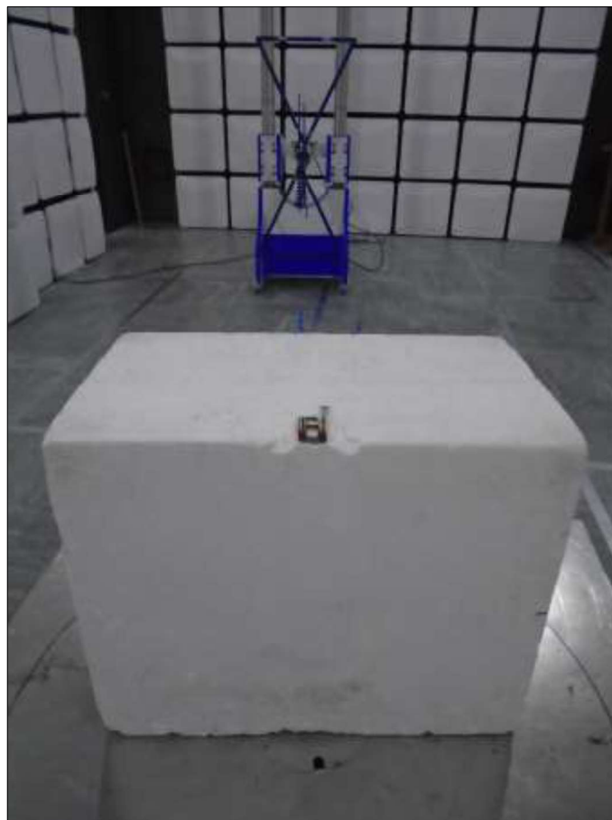
Figure 63 - Test Setup - 30 MHz to 1 GHz - X Orientation
