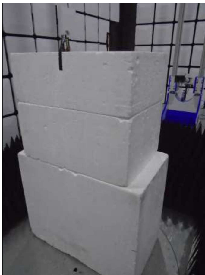
Figure 67 - Test Setup - 1 GHz to 10 GHz - Y Orientation
