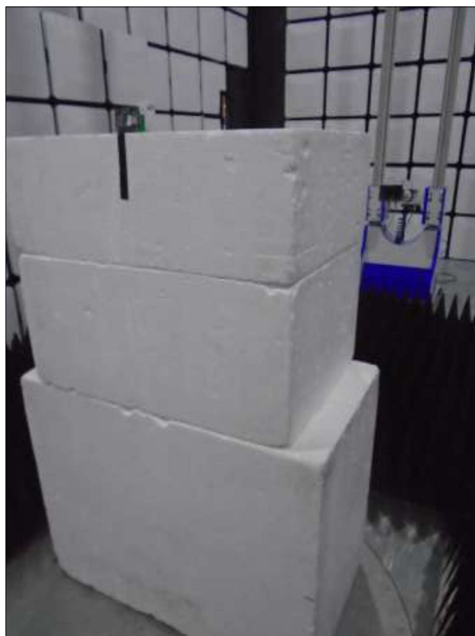
Figure 68 - Test Setup - 1 GHz to 10 GHz - Z Orientation
