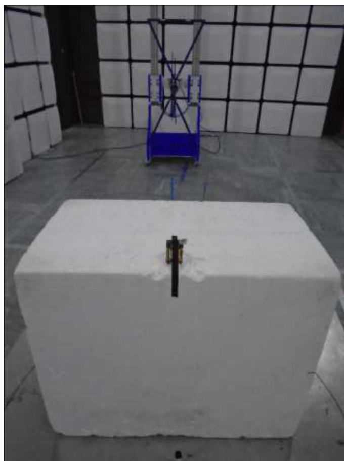
Figure 64 - Test Setup - 30 MHz to 1 GHz - Y Orientation
