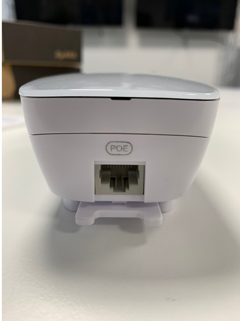
Figure 4: Photo of the POE (power over ethernet) port of the PN 100590 Cloud Connector US
