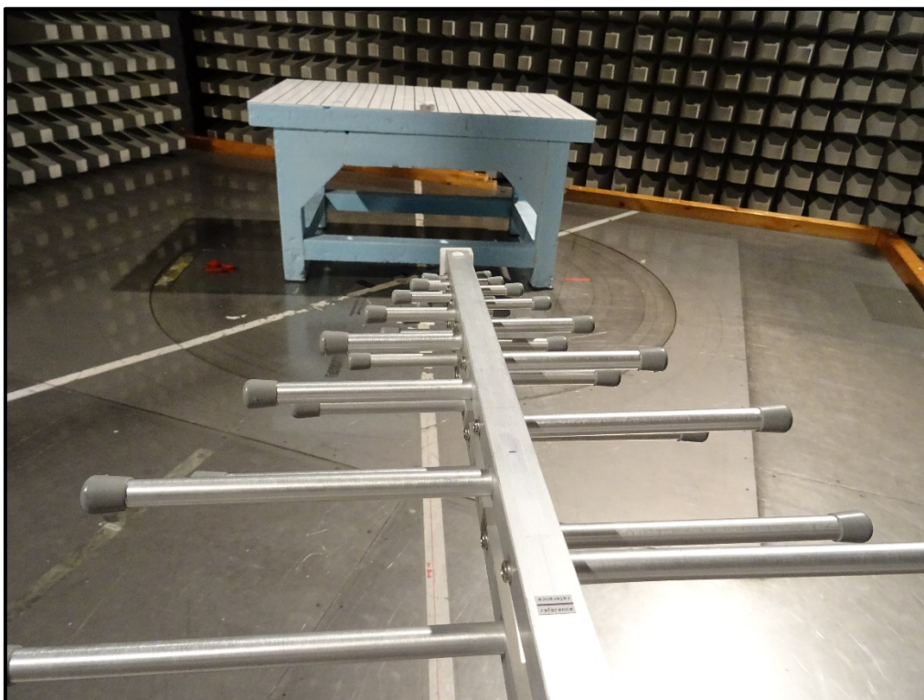
Photo 5: Radiated Test Setup -30 MHz to 1GHz EUT
