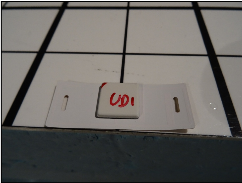
Photo 6: Radiated Test Setup -30 MHz to 1GHz EUT
