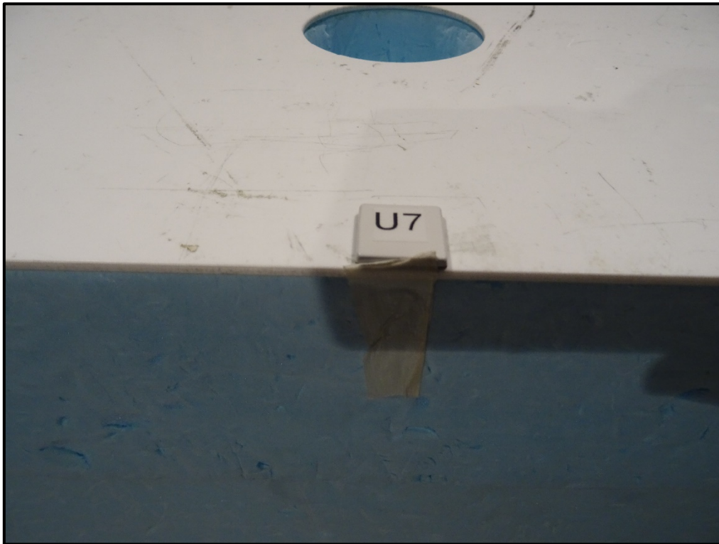
Photo 6: Radiated Test Setup -30 MHz to 1GHz EUT
