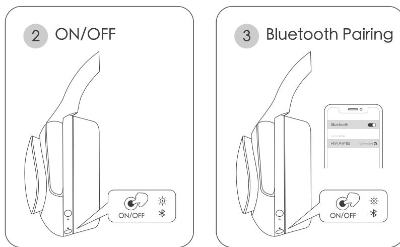
Press and hold the ON/OFF button for 1 second to turn on or turn off the headphone.
