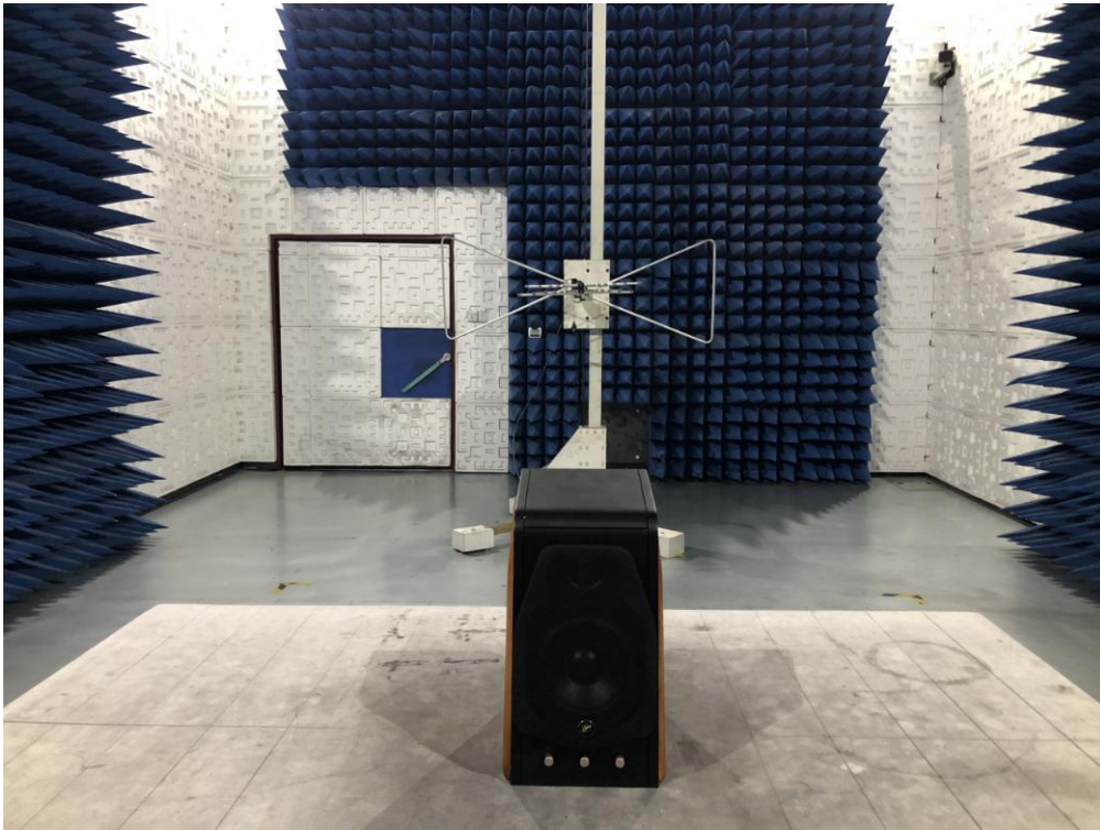
RADIATED EMISSION TEST SETUP ABOVE 1GHz
