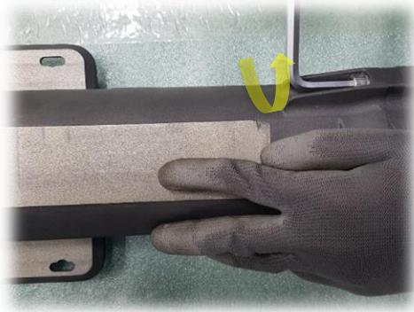
③ Please remove the bolts(M8) which is clamped with BLDC Motor and Jet Tunnel using the hex keys wrenches in a counterclockwise direction.
