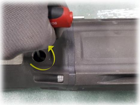
② Please remove the setscrew(M4) which is clamped with the coupling using the hex keys wrenches in a counterclockwise direction
