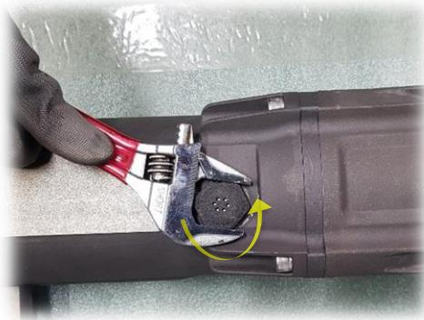
① Please remove the vent-plug using a spanner.
