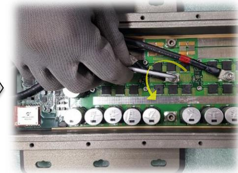
Using the hex keys wrenches in a counterclockwise direction , separate the bolts(M4) which is clamped with U,V, and W-lines.
