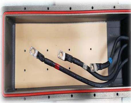
⑥ Before closing the cover, you should put a rubber packing. Please remove the original PCB and replace a new PCB. For assembling, Do it in reverse order
