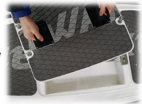
① To unlock them, please turn 4 Fasteners at 180 degrees in a counterclockwise direction.
