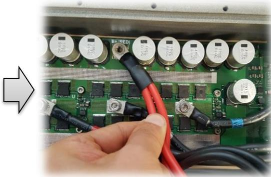
② Please separate the bolts(M5) which are connected with red line(+) and black line(-) in a counterclockwise direction
