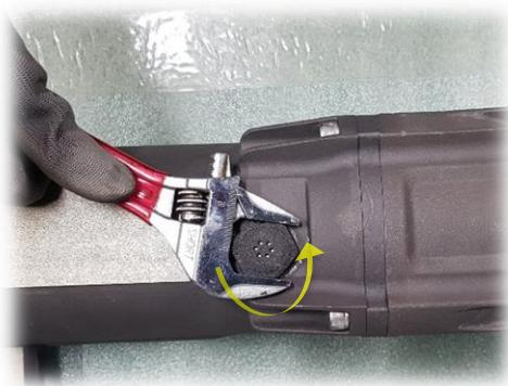
① Please remove the vent-plug using a spanner.
