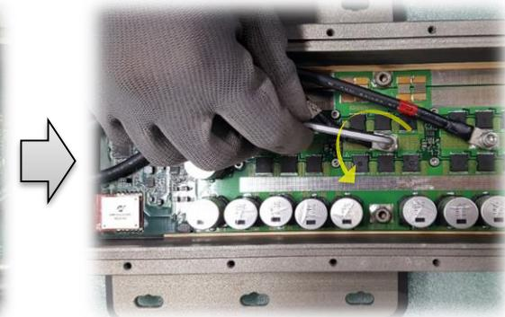
Using the hex keys wrenches in a counterclockwise direction , separate the bolts(M4) which is clamped with U,V, and W-lines.
