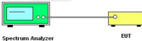
The EUT is connected to the Spectrum Analyzer; the RF load attached to the EUT antenna terminal is 50Ohm; the path loss as the factor is calibrated to correct the reading. Make the measurement with the spectrum analyzer's resolution bandwidth (RBW) = 100 kHz. In order to make an accurate measurement, set the span greater than RBW.
