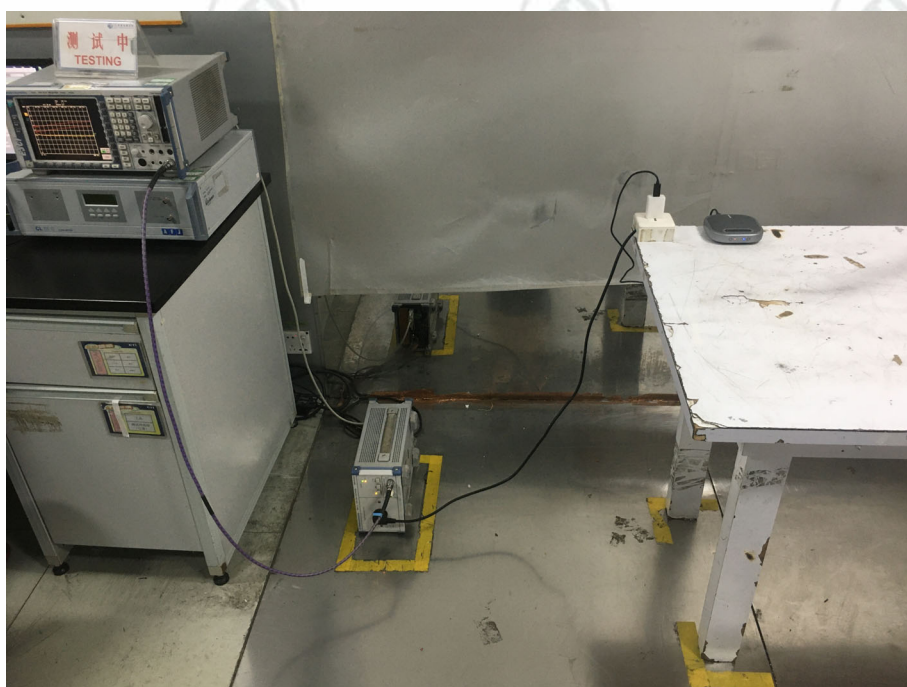
Radiated spurious emission Test Setup-2(CE)
