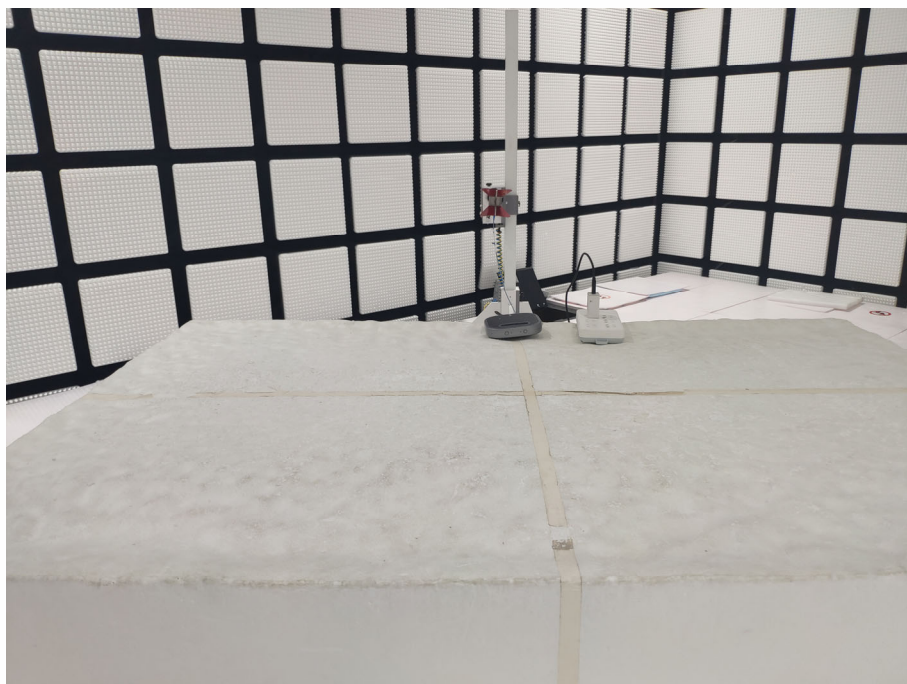
Radiated spurious emission Test Setup-2(Above 1GHz)
