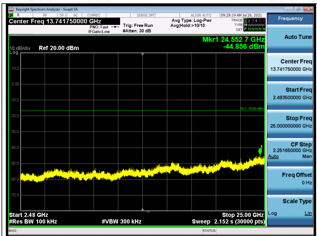
Test_Graph_EDR_ANT1_2402_3Mbps_Higher Band Emissions
