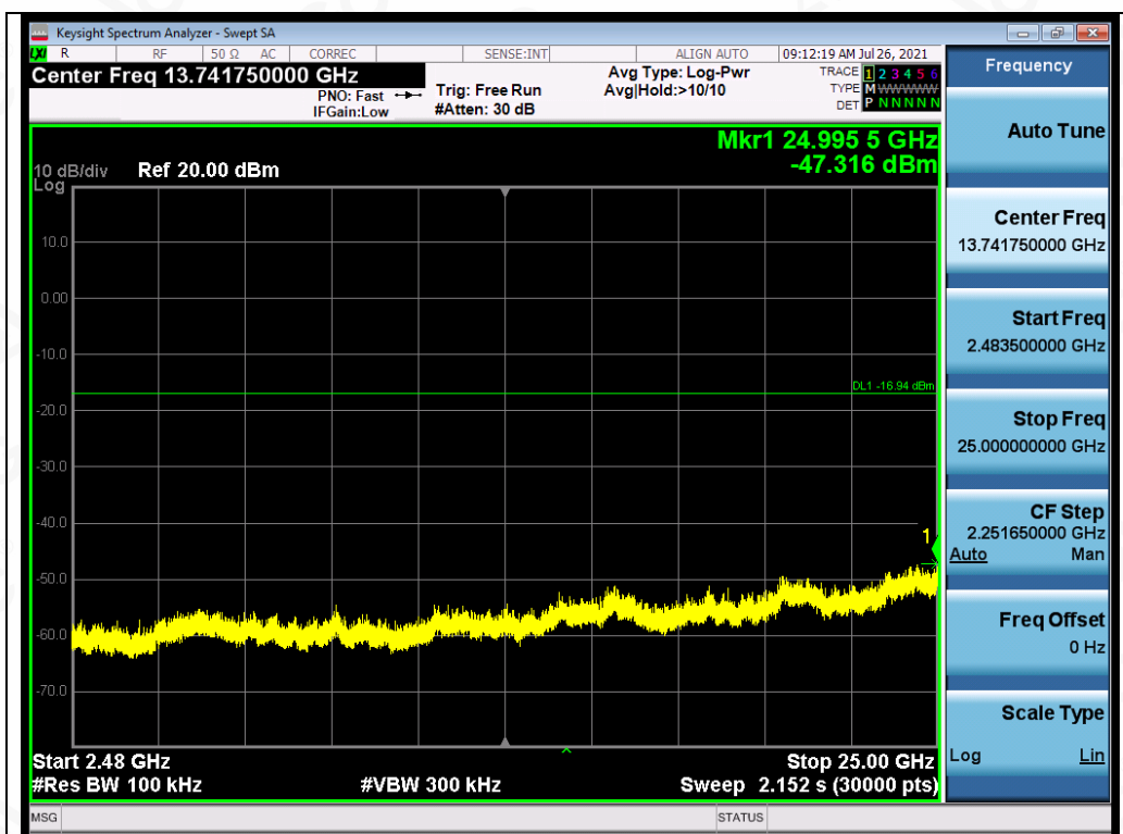
Test_Graph_EDR_ANT1_2441_2Mbps_Higher Band Emissions
