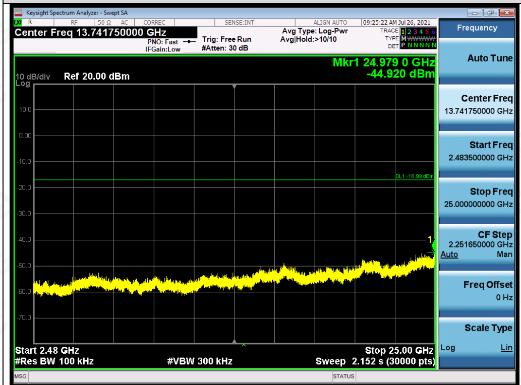
Test_Graph_EDR_ANT1_2402_2Mbps_Higher Band Emissions
