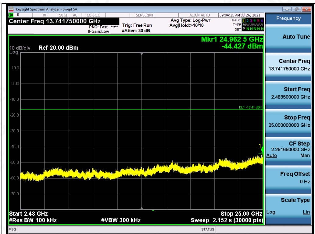
Test_Graph_BR_ANT1_2402_1Mbps_Higher Band Emissions
