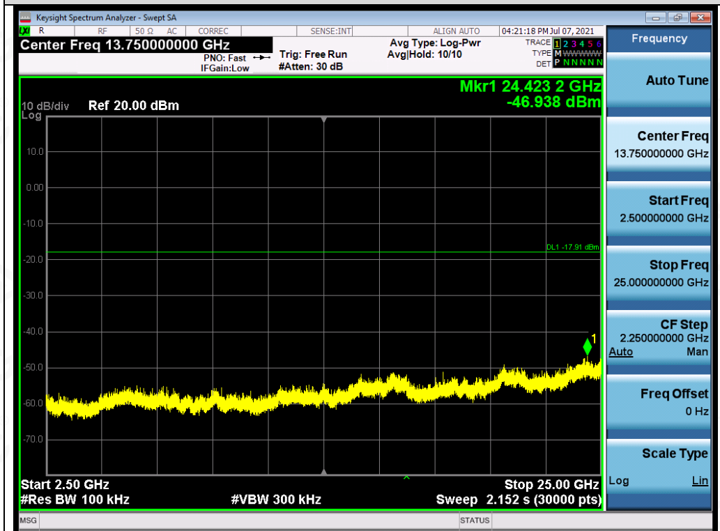
Test_Graph_802.11g_ANT1_2462_6Mbps_Higher Band Emissions
