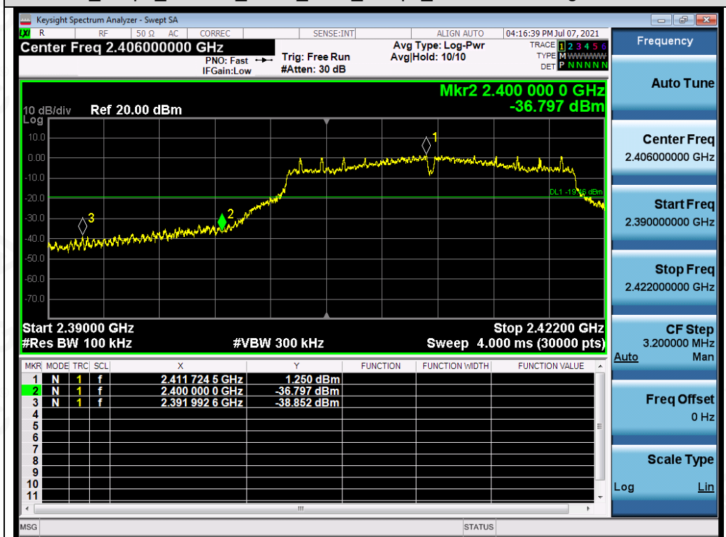
Test_Graph_802.11g_ANT1_2412_6Mbps_Lower Band Edge Emissions
