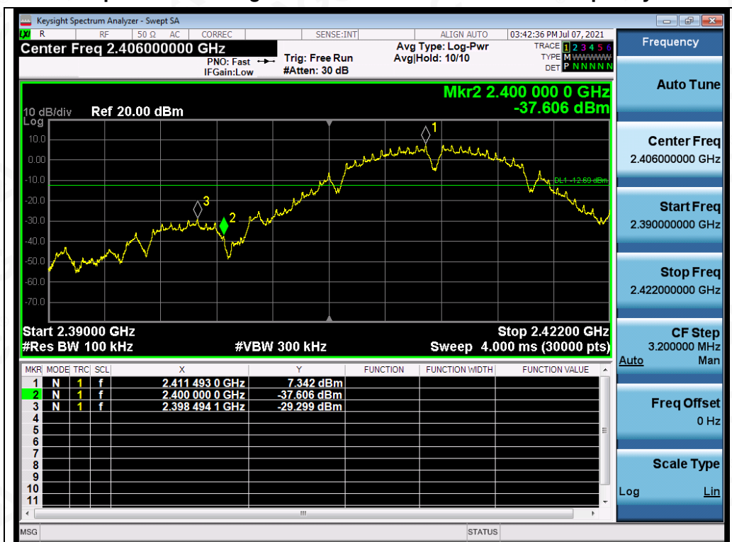
Test_Graph_802.11b_ANT1_2412_1Mbps_Lower Band Edge Emissions
