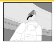
Install outer sensor on tire valve in order
