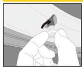
Remove tire valve cap, put in Anti-theft screws
