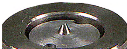
Example of a damaged probe tip (broken tip)
