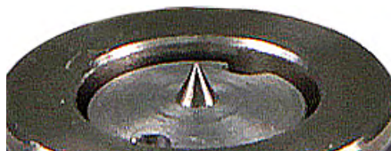
Measuring probe with undamaged probe tip
