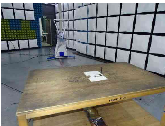
Photo 3: Test setup for radiated measurements (semi anechoic chamber, CFR 47 Part 15, Subpart C)
