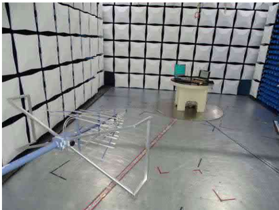
Photo 5: Test setup for radiated measurements (semi anechoic chamber, CFR 47 Part 15, Subpart B, 30 MHz – 1GHz)
