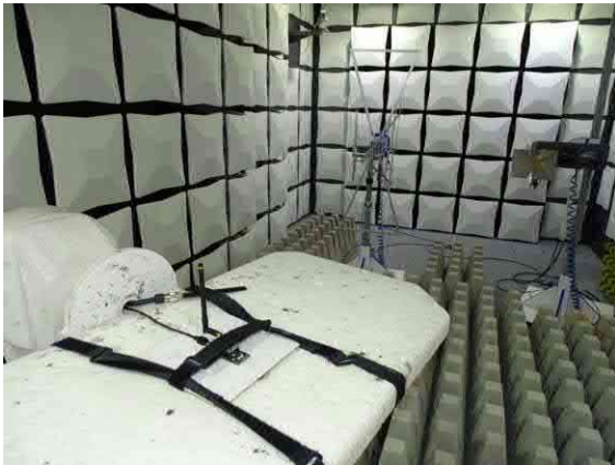
Photo 1: Test setup for radiated measurements (fully anechoic chamber, CFR 47 Part 15, Subpart C)
