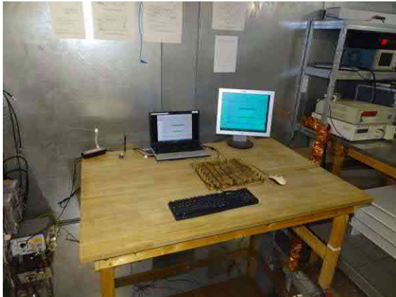
Photo 4: Test setup for conducted measurements (anechoic chamber, CFR 47 Part 15, Subpart B)
