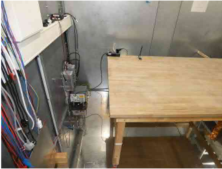
Photo 7: Test setup for conducted measurements (anechoic chamber, CFR 47 Part 15, Subpart C)
