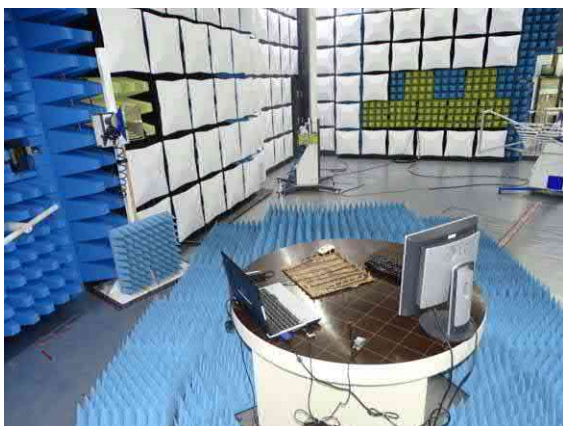
Photo 6: Test setup for radiated measurements (semi anechoic chamber, CFR 47 Part 15, Subpart B, above 1 GHz)
