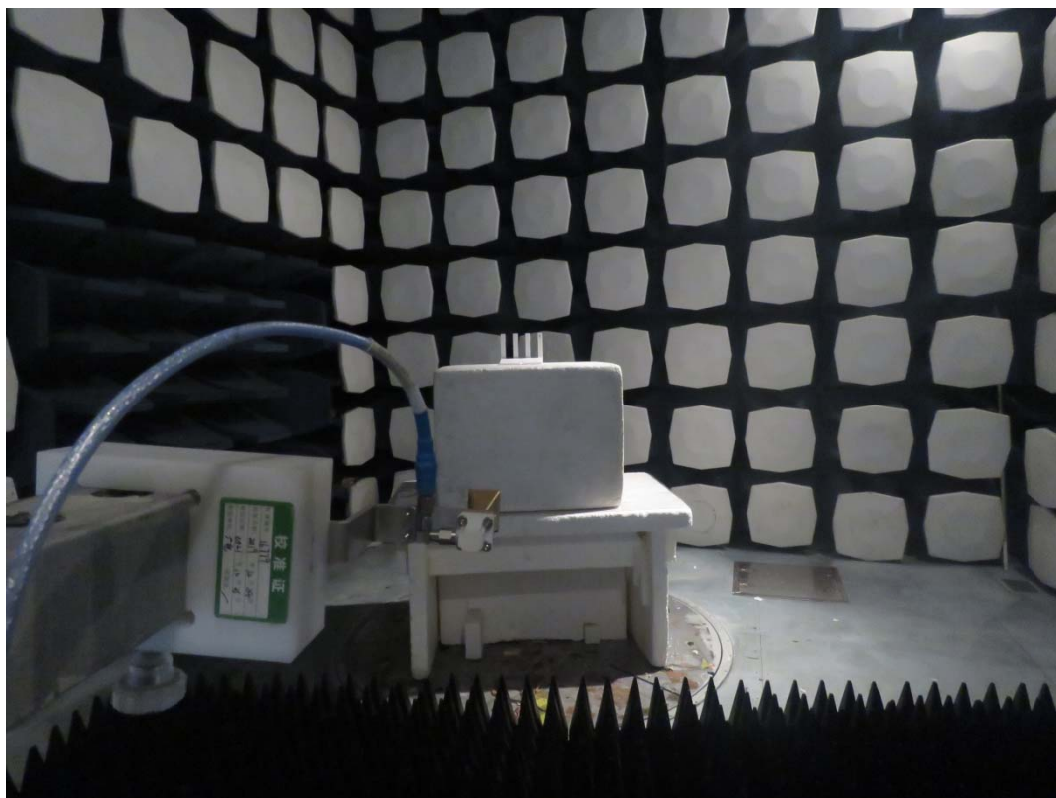
Picture 1 Radiated Emission Test Setup
