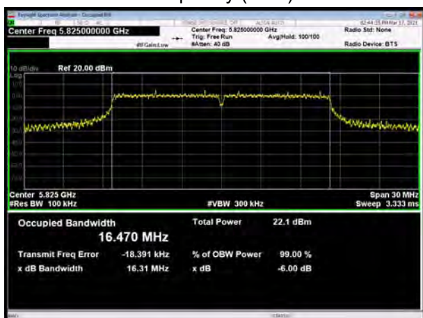
U-NII-3, 802.11n HT40 Carrier frequency (MHz): 5755
