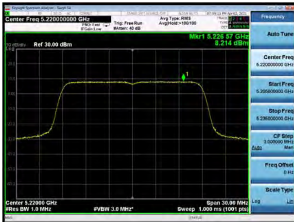
U-NII-1, 802.11ac VHT80, Channel No.: 42
