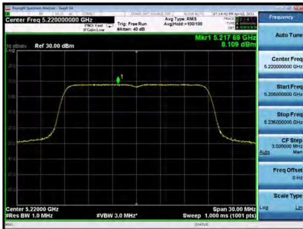
U-NII-1, 802.11ac VHT80, Channel No.: 42
