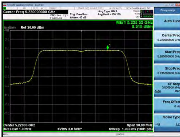
U-NII-1, 802.11ac VHT80, Channel No.: 42
